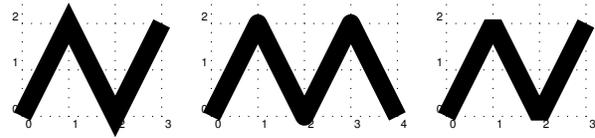
Figure 11: Meaning of the PostScript command `setlinejoin=0|1|2`
